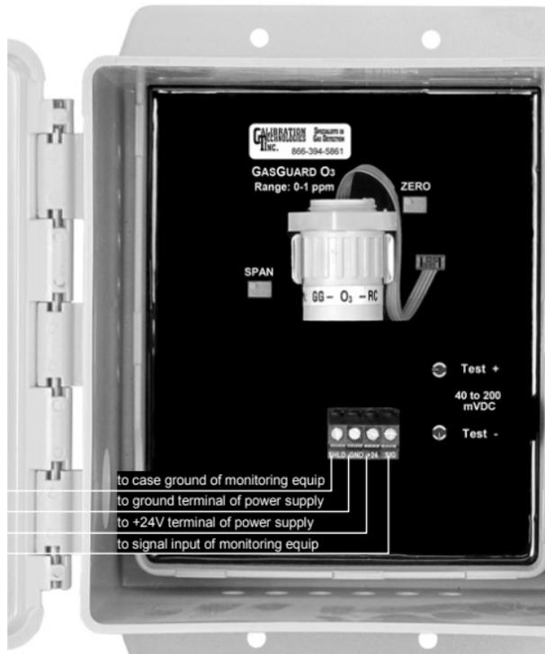
Figure 2: Wiring diagram
