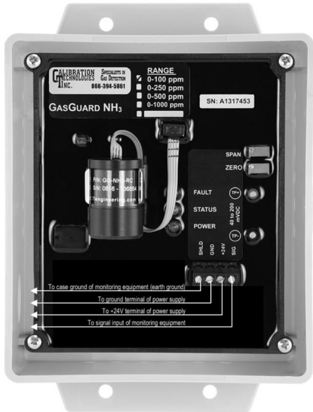
Figure 2: Wiring diagram
