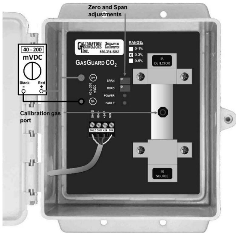
**Figure 3: Sensor output and zero/span adjustments**
