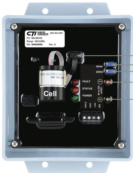
Figure 2: Sensor board components and zero/span adjustment
