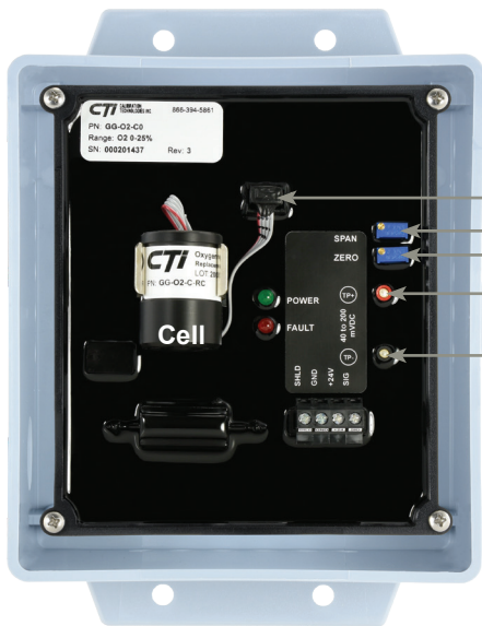
Figure 2: Sensor board components and zero/span adjustment
