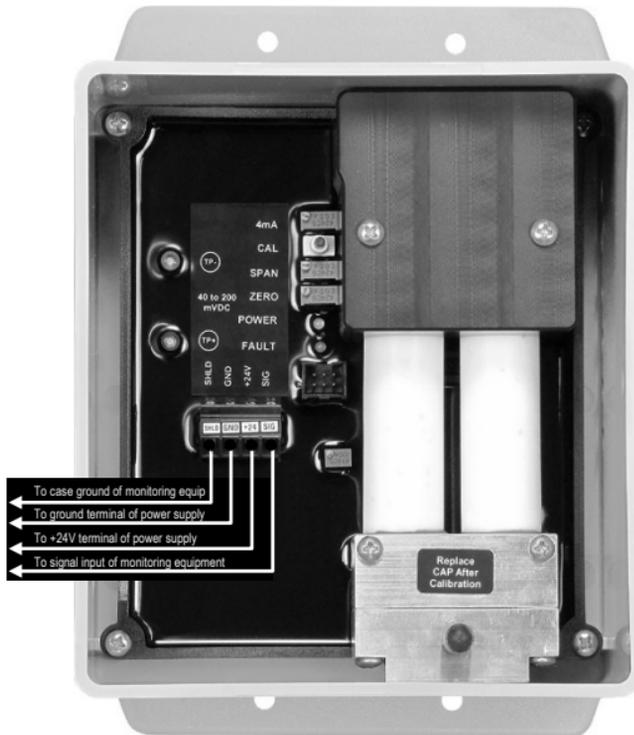
Figure 2: Wiring diagram
